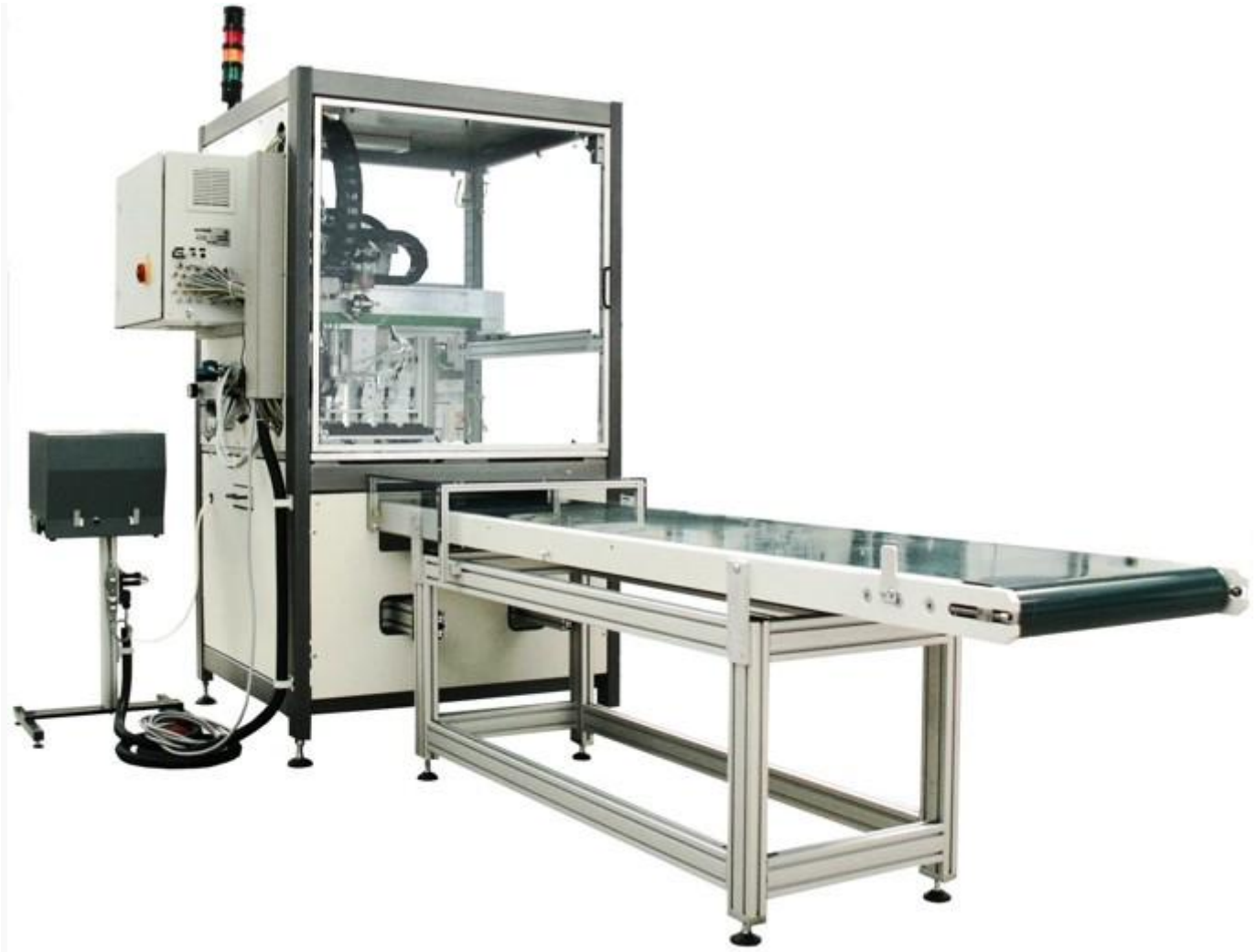
This conveyor connects this Screwdriving Cell with the next Station in the assembly line
