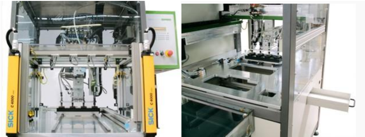
Load Station in the front; Screwdriving Station in the rear
