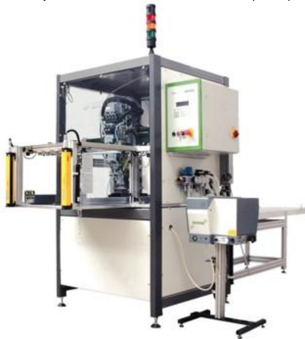
View of the DEPRAG DCAM incl. stationary Screwfeeder
